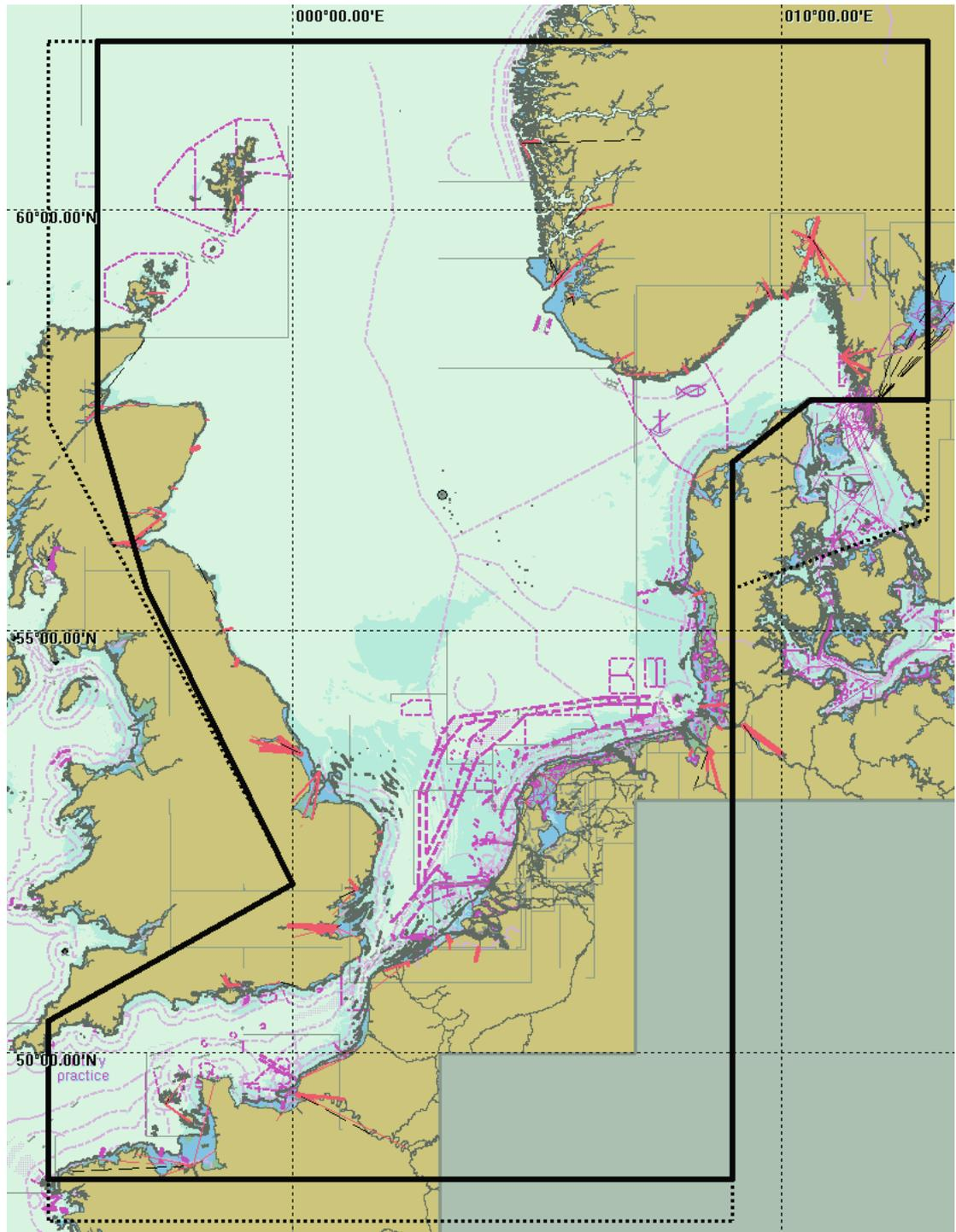
Figure 4-3 Links of the traffic database from sea to port, Dutch ports excluded
