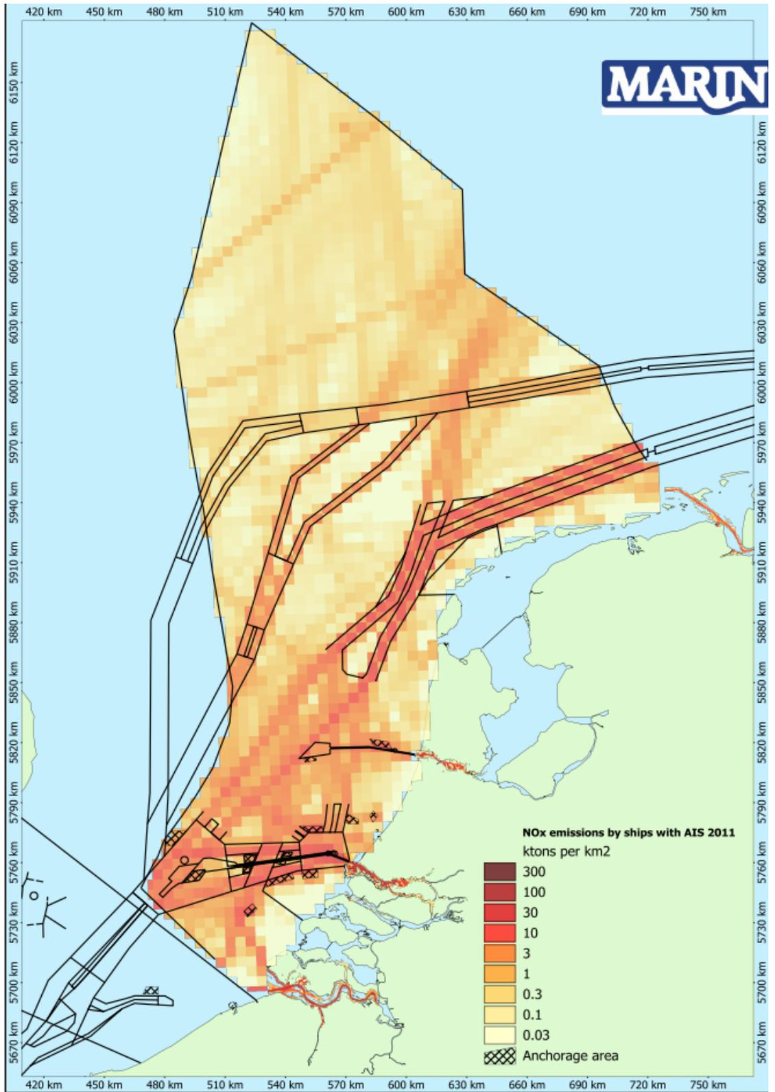
**Figure 8-9** NO<sub>x</sub> emission in 2011 at the NCS and in the Dutch port areas by ships with AIS
